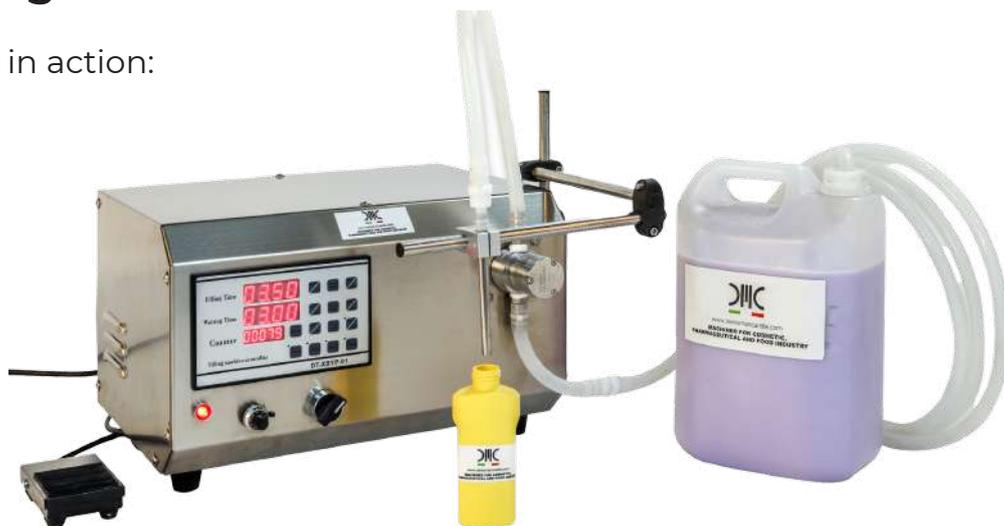
Direct loading from storage tank or barrel
