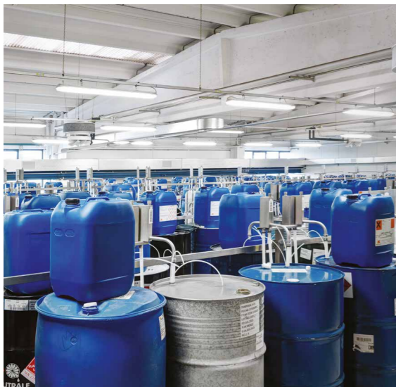
Mezzanine with feeding infrastructures, called the “feeding mezzanine,” serving the automatic compounding system situated on the lower floor. The direct connection of drums can be seen (from drums to dosage line without passage through any hopper) along with the tubing for the nitrogen blanketing necessary to protect the raw materials from oxidation in the halved containers.
