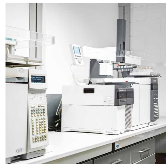
GC/MS system equipped with a PAL-type autosampler (thermostated trayholder and robotic vial processing; static head space; SPME extraction; liquid injection).
