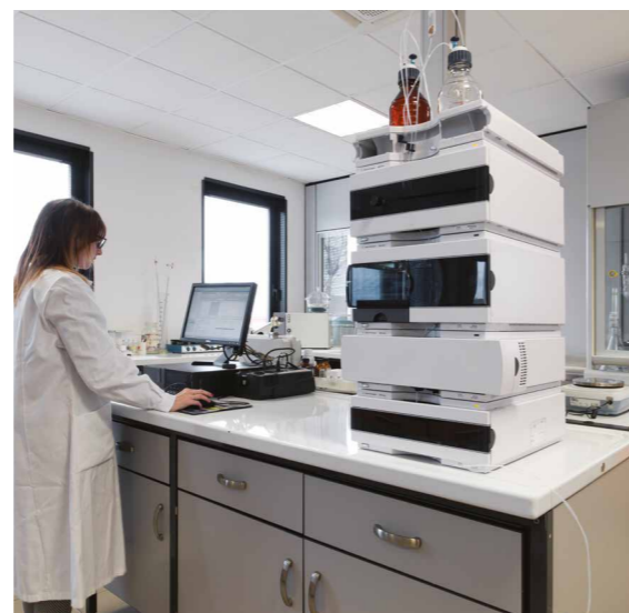
HPLC system equipped with UV-DAD detector and a preparative type autosampler.
