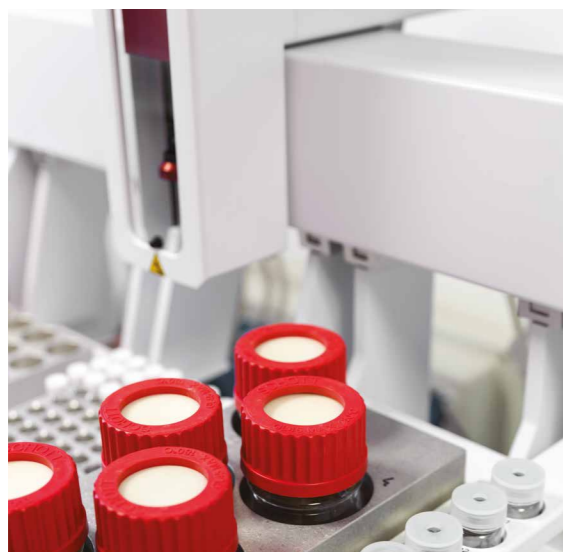
Detail of a Flash GC-based "electronic nose-type" analytical system for the parametric/comparative characterization of olfactory profiles (through multivariate statistics), both of fragrance compounds and other materials (>14,000 in the corporate library). In the foreground, 20-ml vials for "head space" on large liquid volumes or significantly sized solids.
