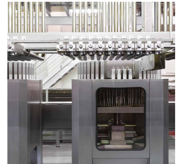
Element of the liquid dosing and mixing line working in the minimum automated weighting range, with 700 different liquids. Through the compartment’s transparent closure, in the foreground, the circular arrangement of the nozzles is visible, under which moves a rotating arm with a scale.
